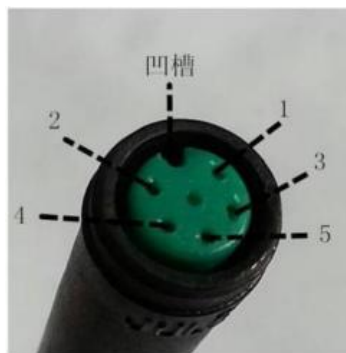
Controller to Display
